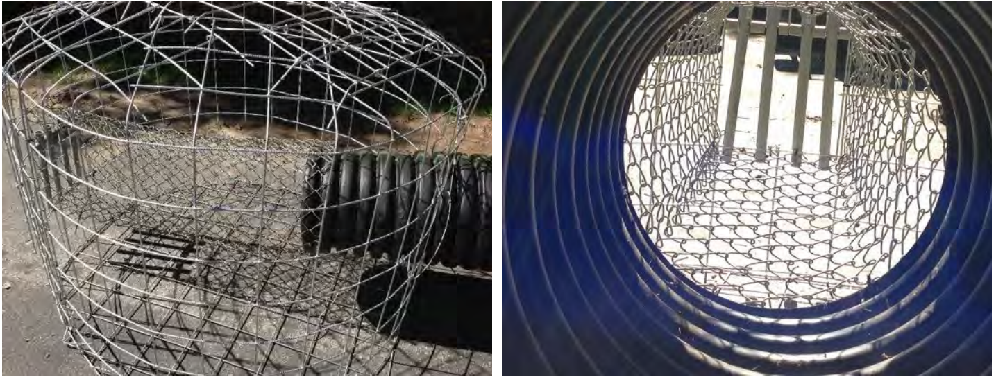
Figure 3. Examples of a modified flexible pond leveller with a one-way fish gate (images from the Beaver Institute).
